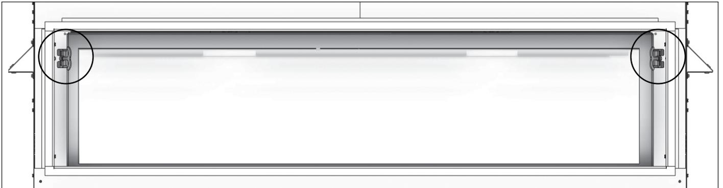
3. Using your finger, pull the lever towards you and unhook it from the window frame bracket.
